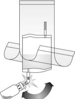
5. Pump the liquid into the vial, but do not fill the vial completely. If flow is not possible, turn the vial again 2 times completely in the same direction to assure that the septum is completely penetrated. Repeat this step until flow is possible.
