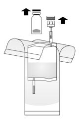
3. Place the BCG-medac vial on a solid surface (e.g. table) and press the adapter of the instillation system upright and firmly onto the BCG-medac vial. Turn the vial 2 times completely in the same direction.
