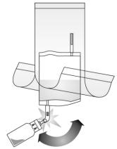
5. Pump the liquid into the vial, but do not fill the vial completely. If flow is not possible, turn the vial again 2 times completely in the same direction to assure that the septum is completely penetrated. Repeat this step until flow is possible.
