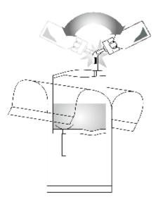
5. Pump the liquid into the vial. Please ensure that the vial is not completely filled!
