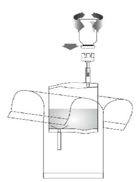
4. Break open the mechanism in the tube of the adapter by repeated bidirectional bending. This establishes the connection. Please hold the tube – and not the vial – during this process!
