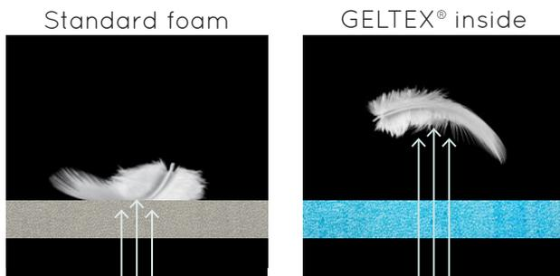
Our laboratory testing demonstrates when using the same pressure of air through the materials the feathers are easily blown into the air through the GELTEX<sup>®</sup> inside material compared with the standard foam.
