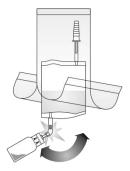
Break open the mechanism in the tube of the connector by repeated bidirectional bending. This establishes the connection. Please hold the tube – and not the vial – during this process!
